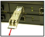
Figure 29: SFP Removal
